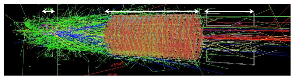
A signal electron, together with all the other interactions occurring simultaneously, integrated over 500-1695 ns window
