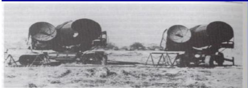
Figure 10.1 The first stellar intensity interferometer; the pilot model of the stellar intensity interferometer at Jodrell Bank in 1955. Two Army searchlights were used to make the first measurement of the angular diameter of a main sequence star (Sirius).
