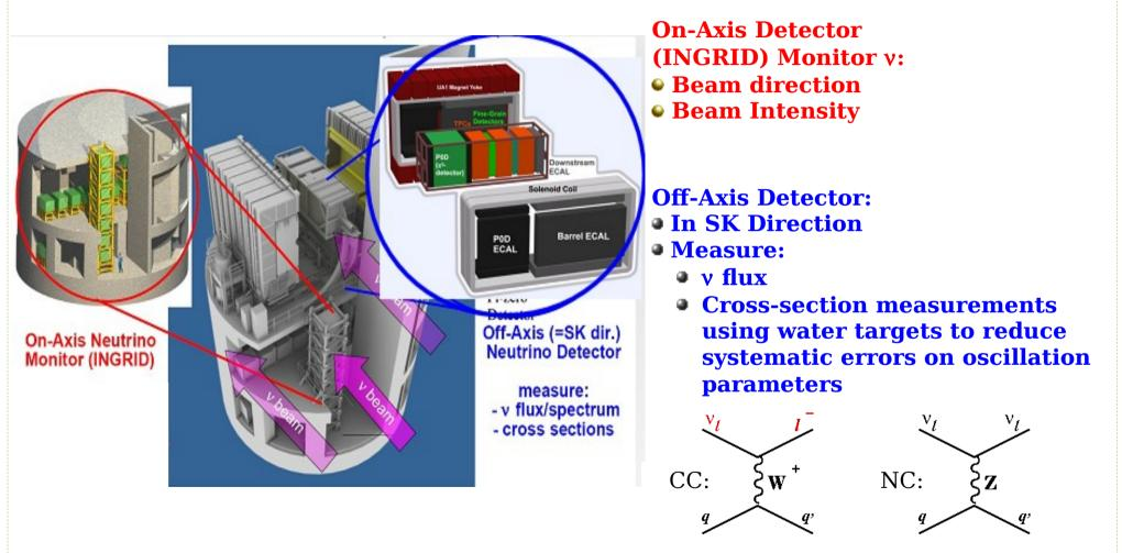
$\rightarrow$  Used for monitoring of beam, flux constraints and systematic error reduction
