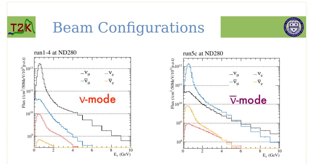
v – mode known as "forward horn current" (FHC) or "positive focusing" (PF)  $\overline{v}$  – mode known as "reverse horn current" (RHC) or "negative focusing" (NF)
