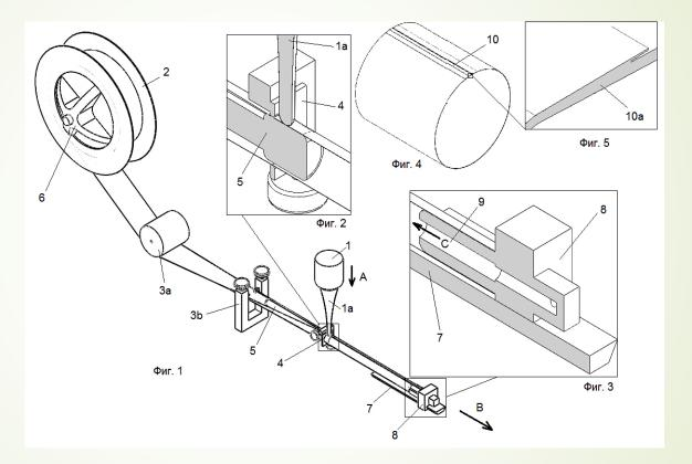
Block – scheme of welding machine. Welding element – sonotrode, 1a.
