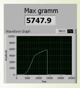
Test bench for checking of seam breaking force: 1 – stress gauge, 2 – sample, 3 – tensioning mechanism User interface for data presentation. Requirements – breaking force should be higher then 4 kg.
