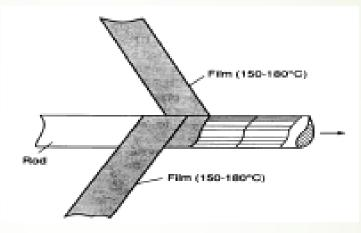
Thickness is two layers of film + glue layer. Glue provides increased straw creep Compared to creep of film`s material. Film is heated to 50 – 70 degree.
