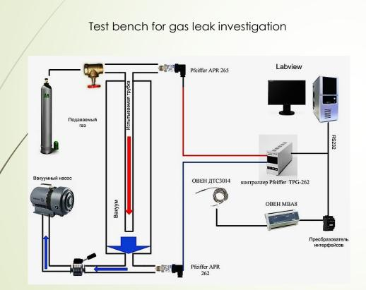
Gas leak of straw 2.5 m. long: Leakage at overpressure 1 atm. Is  $3 \cdot 10^{-4} \ cm^3/min$
