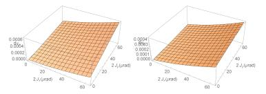
Figure: Amplitude dependent tune shift due to lattice nonlinear magnets in J-PARC MR.
