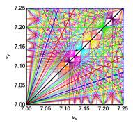
Figure: .Tune diagram near  $(\nu_x/3, \nu_y/3) = (7.13, 7.143)$ , where total tune is (21.35, 21.4).
