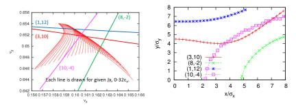
Figure: Tune spread area and resonance in the amplitude space for a hadron collider, SPPC (x-crossing), long range collisions are included.
