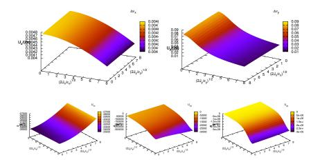
Figure: Tune spread and slope in SuperKEKB (detuned  $\beta_v = 3$  mm).
