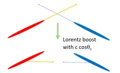
Figure: Schemetic view for crossing collision (K. Oide, PRA40, 315(1989), K. Hirata, PRL74, 2228 (1995)).
