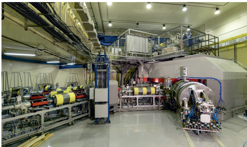
Gas-filled recoil separator of the SHE Factory
