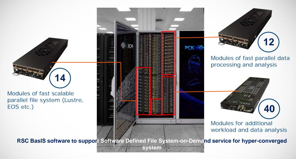
Hyper-converged system allows to use all Storage nodes as computing ones in parallel with store/retrieve data. This will add 230TFLOPS to GOVORUN system, almost doubling the CPU part performance.
