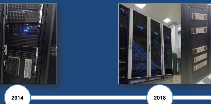
Total peak performance: 140 TFlops for single precision; 50 TFlops for double precision Total peak performance: 1000 TFlops for single precision; 500 TFlops for double precision
