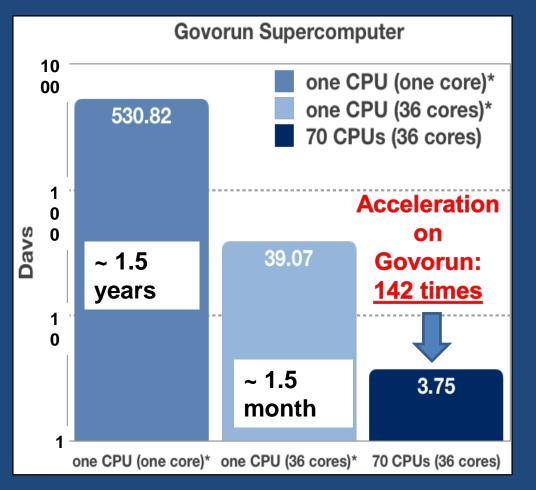
A hybrid algorithm MPI+OpenMP has been developed for solving optimization problem for nonlinear The unsteady heat equation. optimization problem has been formulated in order to improve the design of so-called "temperature valves" technique for the pulse injection (in the millisecond range) of working gases into the multiply charged ion source ionization chamber.
