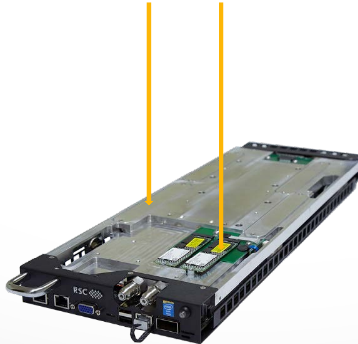
Unified power connectors for easy upgrade/reconfiguration
