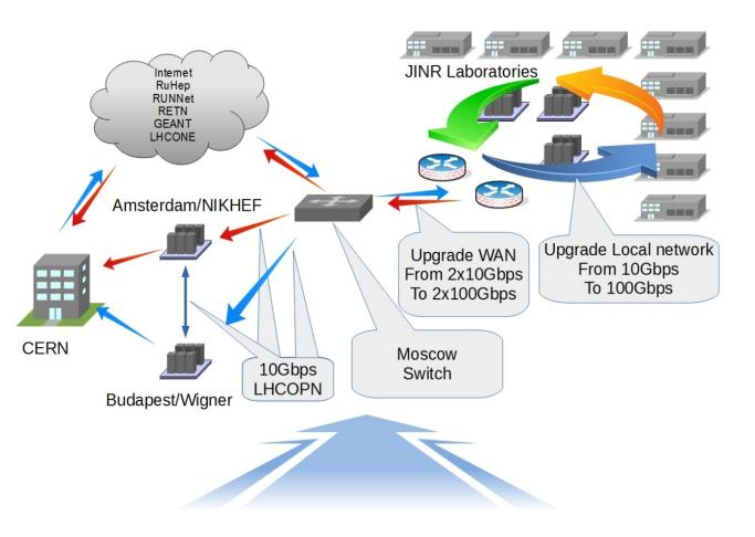
Local Area Network – 2x10 Gbps, planned upgrade to 100 Gbps Wide Area Network – 2x10 Gbps, 100 Gbps Upgrade WAN to n x 100 Gbps planned One of the most important components of JINR and MICC providing access to resources and the possibility to work with the big data is a network infrastructure.
