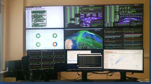
The system allows one, in a real time mode, to observe the whole computing complex state and send the system alerts to users via e-mail, sms, etc. ~ 850 elements are under observation ~ 8000 checks in real time ~ 100 scripts
