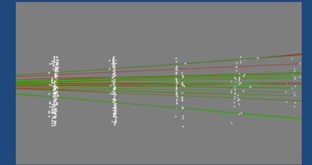
Input data for the first step algorithm were simulated by GEANT in MPDRoot framework for the real BM@N configuration.
