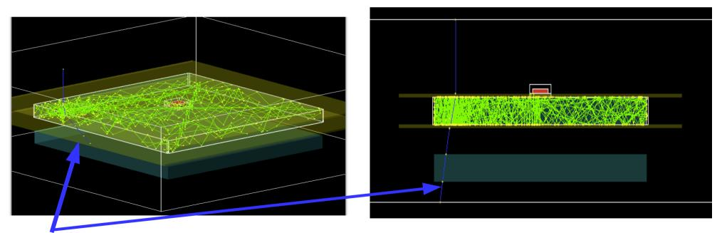
Electron falls vertically. Simulated value of SiPM shift is (0.0, -0.5, -0.95) mm. Optical photons and SiPM located in the center of the tile.
