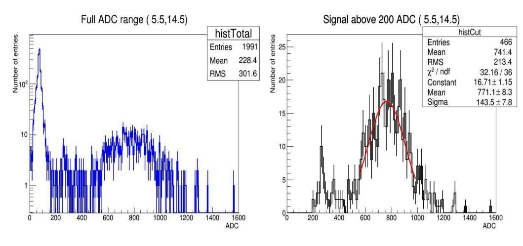
Gaussian fit in the range  $\pm$  1.5 RMS The sophisticated fit procedure was developed to achieve reliable fit results.
