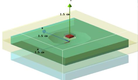
Slab: 40 x 0.2 x 40 mm<sup>3</sup> Thickness of foil is 65 microns Epoxy: 3 x 0.4 x 4 mm<sup>3</sup> Trigger tile below measured tile Wrapping foil not shown
