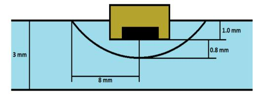
Tile:  $30 \times 3 \times 30 \text{ mm}^3$ SiPM box:  $3.8 \times 1 \times 3.8 \text{ mm}^3$ SiPM:  $2.2 \times 0.5 \times 2.2 \text{ mm}^3$ (schema not to scale) reflective foil: 40 x 0.4 x 40 mm<sup>3</sup>
