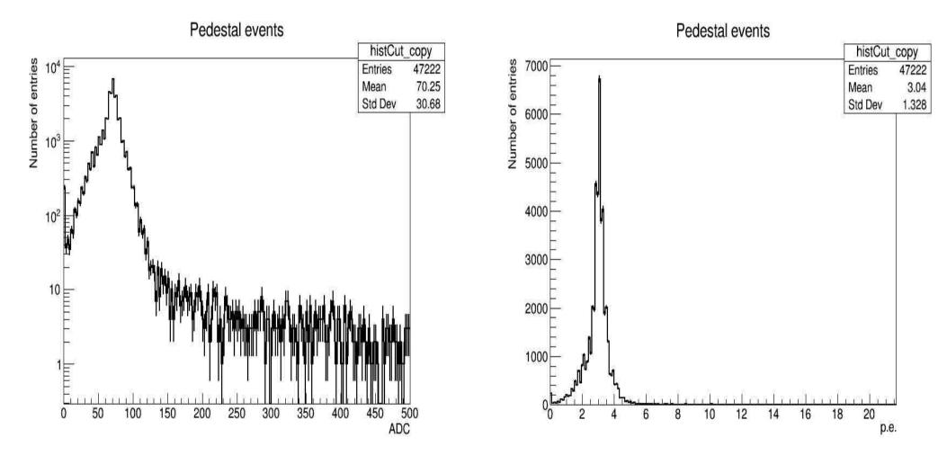
More than 98% of pedestal events are below 200 ADC ( A[p.e.] = A[ADC] / G ). Measured gain G = 23.11 ADC.
