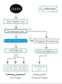
\* As a result of this flow we have 4 spectra for different CVN PID binning and Peripheral sample separately.
