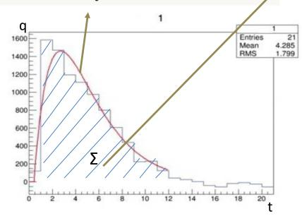
Alternative scheme: Parameterize a maximum value  $(A_{par})$  with a sum signal value at the time( $\Sigma$ ) in each channel.
