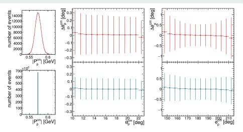
Errors of reconstructed proton momentum in polar coordinates  $(|P_p^{\rm cm}|, \theta_p^{\rm cm}, \phi_p^{\rm cm})$  for the  $pp \to pp$  reaction at ANKE, simulated for  $T_{\rm beam} = 700$  MeV with and without kinematic fitting.
