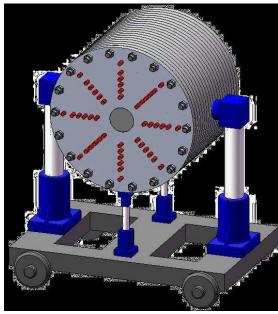
The big uranium target is cylinder from uranium (0/3% 235U). The length of target is 1000 mm, the diameter is 1200 mm. The target put into steel shell with thickness in 100 mm.
