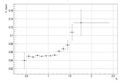
Figure 2: Dependence of the effective temperature T on the variable  $n_c$  for protons.
