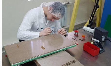
Soldering HV connector and readout pins
