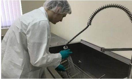
Glass cleaning with ultrasonic wave & deionized water
