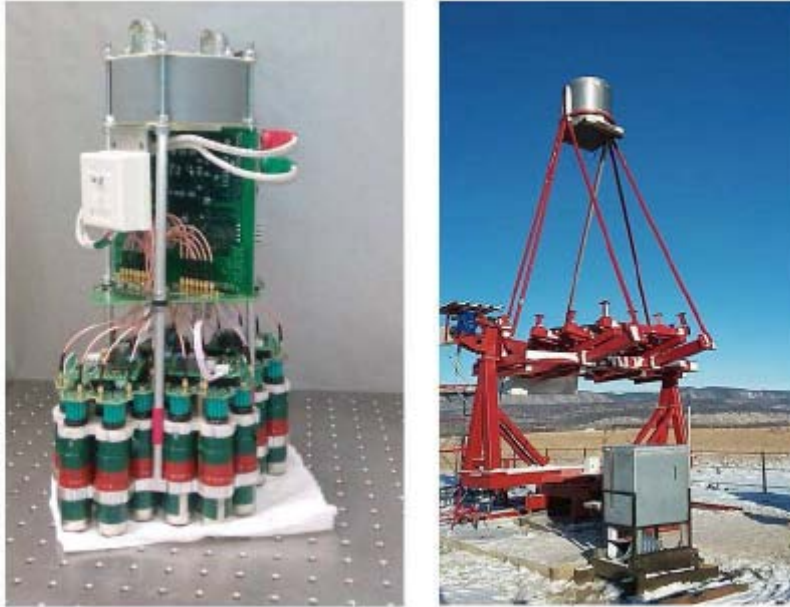
Fig. 3. Left figure: Cluster of 28 PMTs. Right figure: The first TAIGA-IACT.
