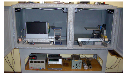
X-ray station for detector calibration
