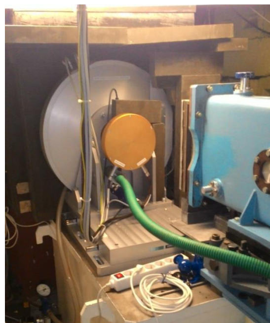
Fig. 40. New mirror neutron guide with vertical parabolic convergence (at left) and new Fourier chopper (at right) in the working position at the HRFD diffractometer.
