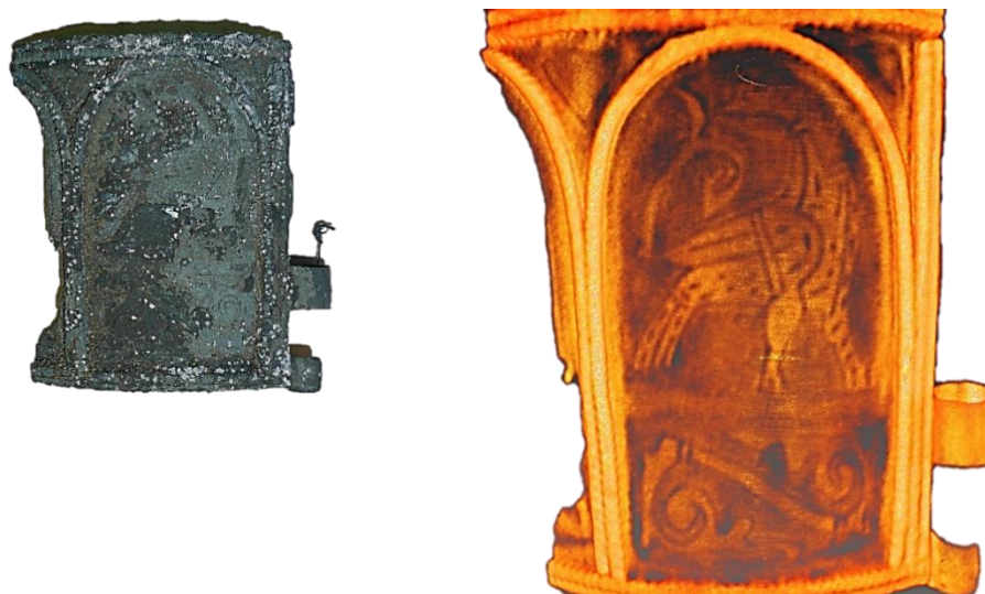
Fig. 35. Photo of a fragment of the ancient bracelet from the treasure found in the city of Tver (left) and its 3D image reconstruction from neutron tomography data (right).
