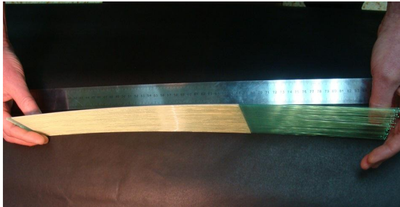
Fig. 2. Element of the scintillation screen (white plate) together with the optical wavelength shifting fibers glued to it on both sides. The curved shape of the screen is determined by the requirement of space-time focusing.
