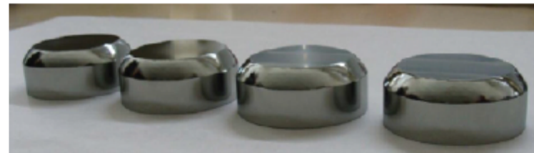
The 4 HPGe point contact 450-g detectors built at JINR.
