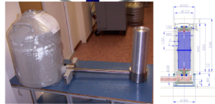
U-type low-background cryostat (left) and the scheme of its detector part.
