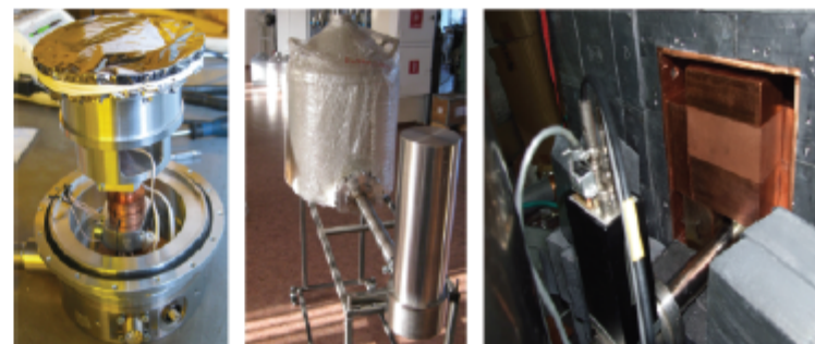
The low background cryostat built by BSI. Internal part; Assembled, test of low radioactive shield at LSM.
