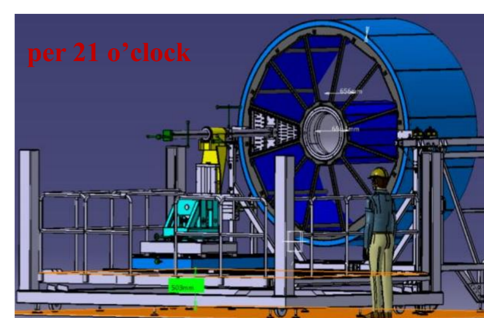
Manipulator for ROC chamber installation
