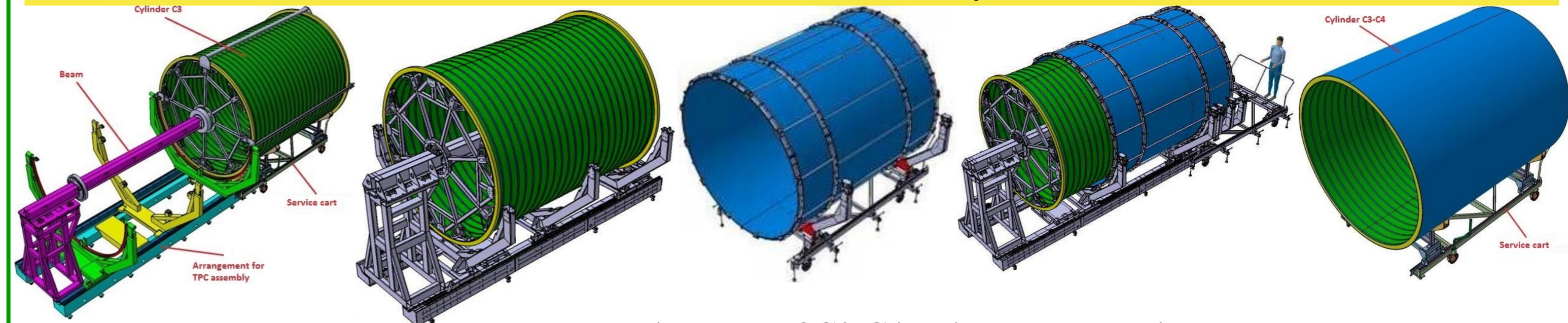
The consecutive steps of C3-C4 cylinders assembling procedure
