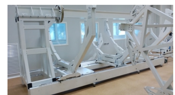
Tooling for TPC assembling in to clean room
